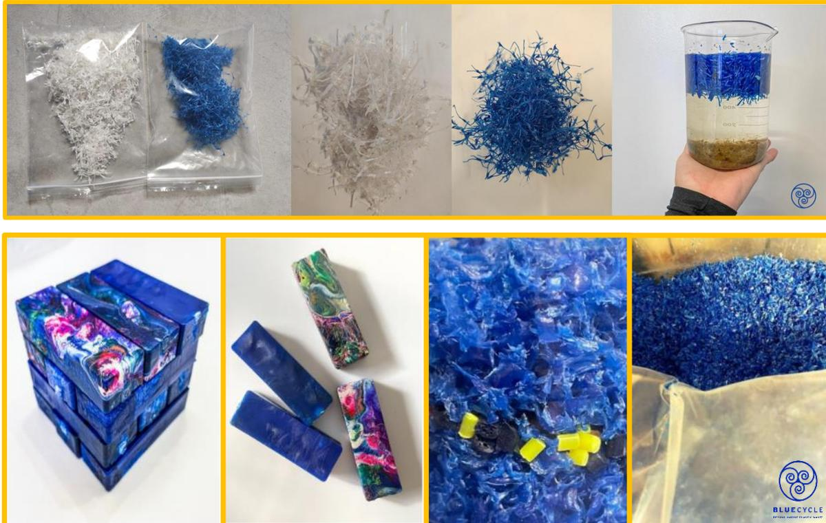
*Figure 4-4. The end product from the mechanical recycling of mussel nets.*
